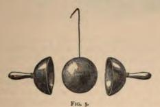
and suspended by a silk thread, and then covered with two hemispherical surfaces of brass, which exactly fit it. When the hemispheres are withdrawn, it will be found that they are charged with electricity, which has been entirely taken from the brass ball.
